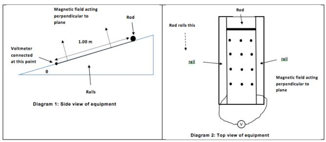
The diagrams below illustrate how the equipment was set up in this experiment.
