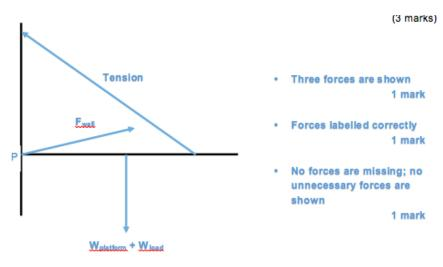
The platform is designed to support a load of 8.5 tonnes and is 15 m long. A single steel cable supports the platform, attached 10.0 m from the end at 55° as shown in the figure. The platform has a mass of 0.7 tonnes.
